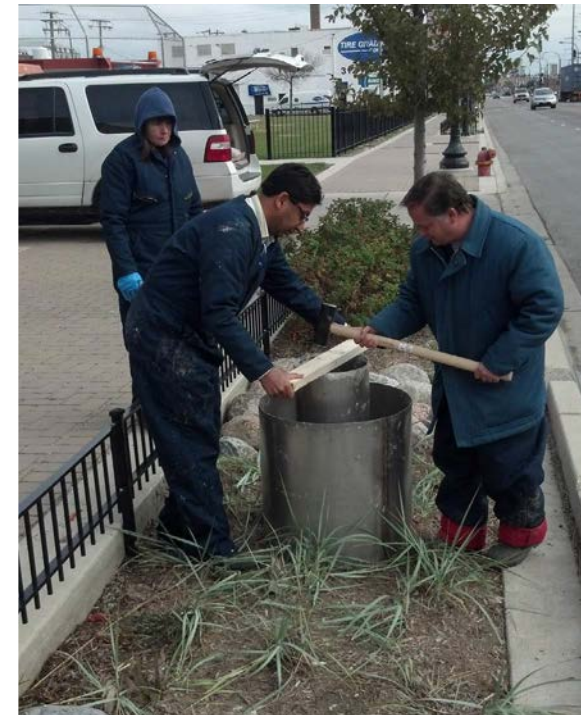
Infiltration Test in Cermak Planter
